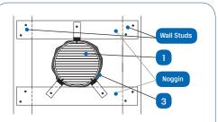
FACE FIXING: Alternative fixing method Kilargo Intumescent fire damper supported by noggins fixed to studs
