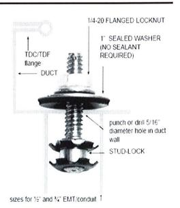
Stud-lock is the result of combining our field tested condu-lock and a threaded stud. This component will allow one person to reinforce duct without assistance. The threaded stud extending out of each end of conduit will allow the installer to easily find pre-drilled holes in both insulated and non-insulated duct.
